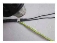
**14.** Before the tube is cold, pinch it at the area between wires with pliers, and hold for 10 seconds to ensure seal.
