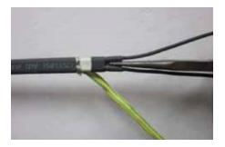
**15.** Final appearance for heating cables with an outer jacket.
