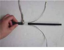
8. Cut off remaining PTC material, leaving the exposed wires. Do not cut bus wires!
