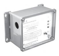
The SST-2 Freeze Protection Thermostat operates from automatically selected operating voltages of 120, 208, 240 or 277 volts, single-phase. They control heater loads of up to 30 amps while consuming less than 2 watts when idling.
